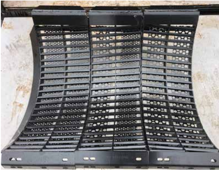
Angled bars, in different directions, improve thrashing
