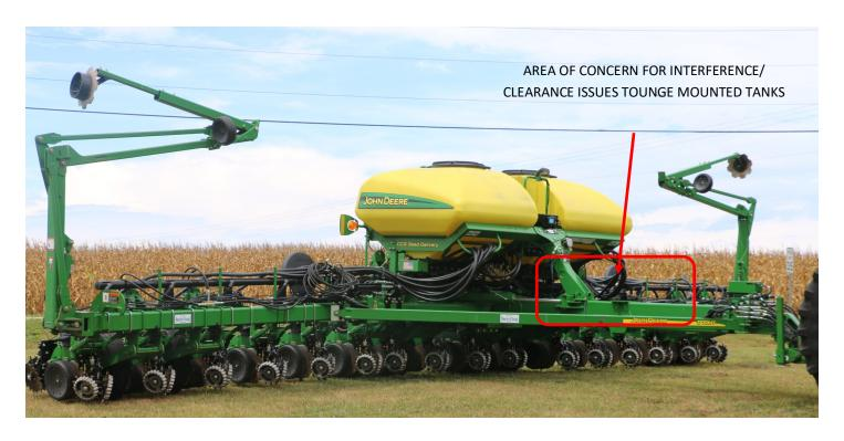
Determine if you will need to use NORMAL or REVERSE mounting methods for the front bracket to avoid Hydraulic fitting bulk-heads, wiring/hose looms, supports or fertilizer tanks.
