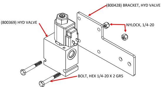
NOTE: VALVE CAN BE ROTATED 90 DEGREES ON THIS BRACKET
