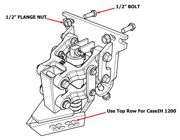
As shown in the picture, Each Stem's side plate has two rows of holes (8 holes total). One of the holes on each side must be selected based on your soil condition and your planter manufacturer to attach the wheel assembly to the stem.
