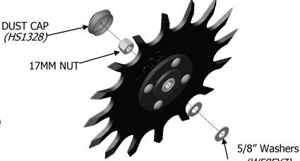
(W58FYZ) (Add as needed to obtain proper spacing)
