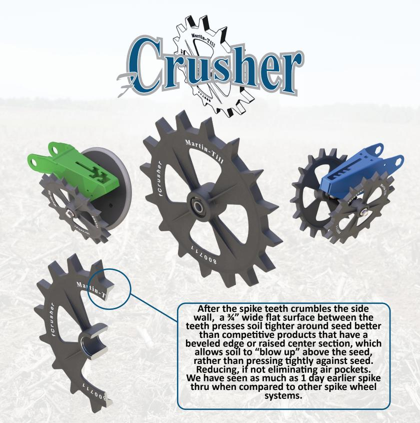
Lightweight (9.5 lbs) cast fCrusher Closing Wheel. Tapered tooth design allows firming on one side and crumbling on the other. Drafted tooth keeps its entire foot print on the ground. No more wearing one side of plastic until it has to be flipped. Long life ductile cast iron will run for years. Martin Duty with PEER Seed Extreme 6 lip seal bearing.
