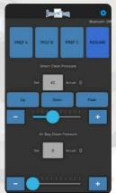
**Dual valve** with one directional control valve works same as single valve plus you can set psi on a second circuit to control air bags.
