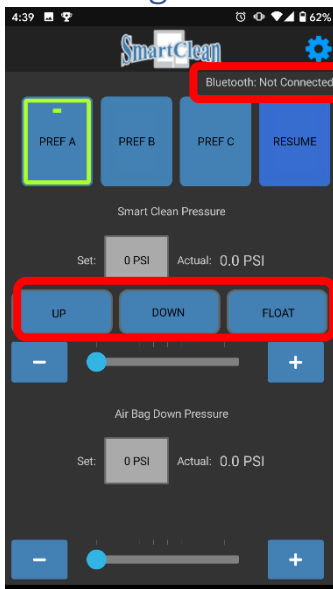
Not Connected State (Bluetooth: Not Connected and UP/DOWN/FLOAT buttons are all blue)
