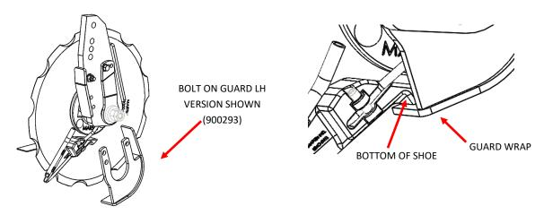
STEP 3): Install the Guard with 3 new 5/16-18 X 1 1/4 bolts and new Flange Nuts included with kit.
