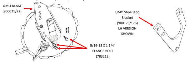
STEP 2): Slide on Guard Assembly as shown below to the inside where the original stop bracket was located . Slide up so that the guard wrap makes contact with bottom of shoe.
